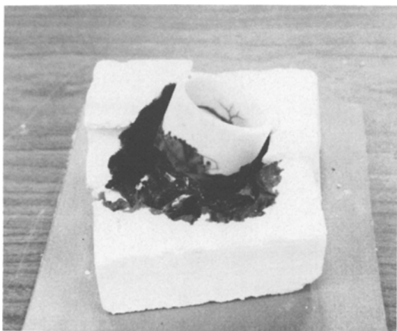
Figure 8 Melted combination of basalt-10% ilmenite rock, alumina crucible, and zircar insulation.
