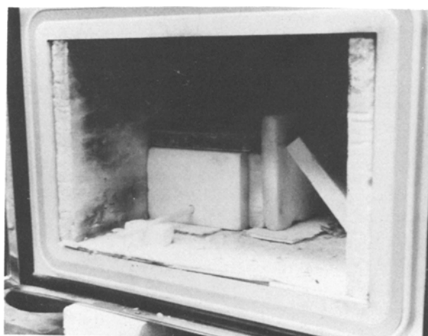
Figure 2 27.62 \times 7.62 cm zircar cavity shaped to fit sample. Alumina tube extends to make optical temperature readings.
