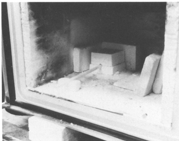
Figure 1 5.08 cm thick zircar cavity built around the sample.
