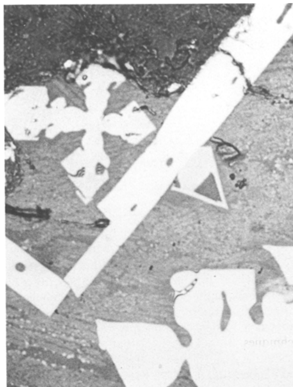
Figure 5 Microwave melted ilmenite rock. Crystals of haematite, ilmenite, and titanomagnetite (cruciform) in glassy silicate matrix.
